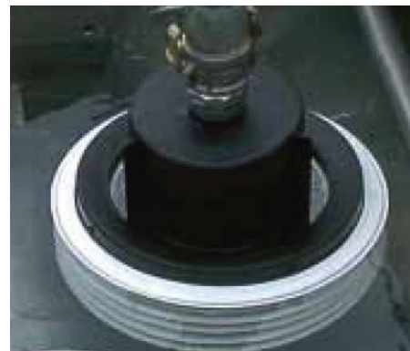
Weir skimmer Terrapin (8.5 kg), 165 dm 3 /min
