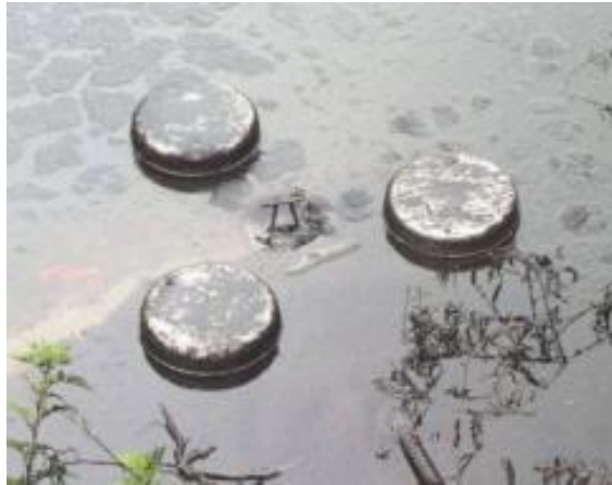
Alpha 1½" weir skimmer (9 kg), up to 150 dm 3 /min
