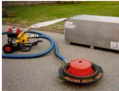
Weir skimmer Mini-Max (22 kg), 510-830 dm 3 /min
