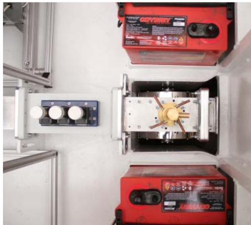
Fig. 5. Part of microwave plasma module with oil-water separator beneath.
