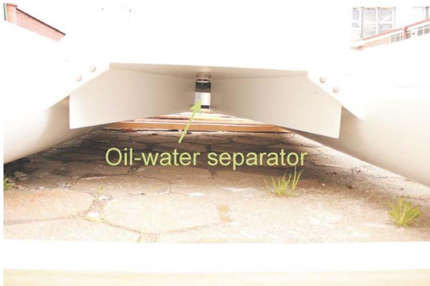
Fig. 6. Bottom view of the floating device showing drivers and oil-water separator.
