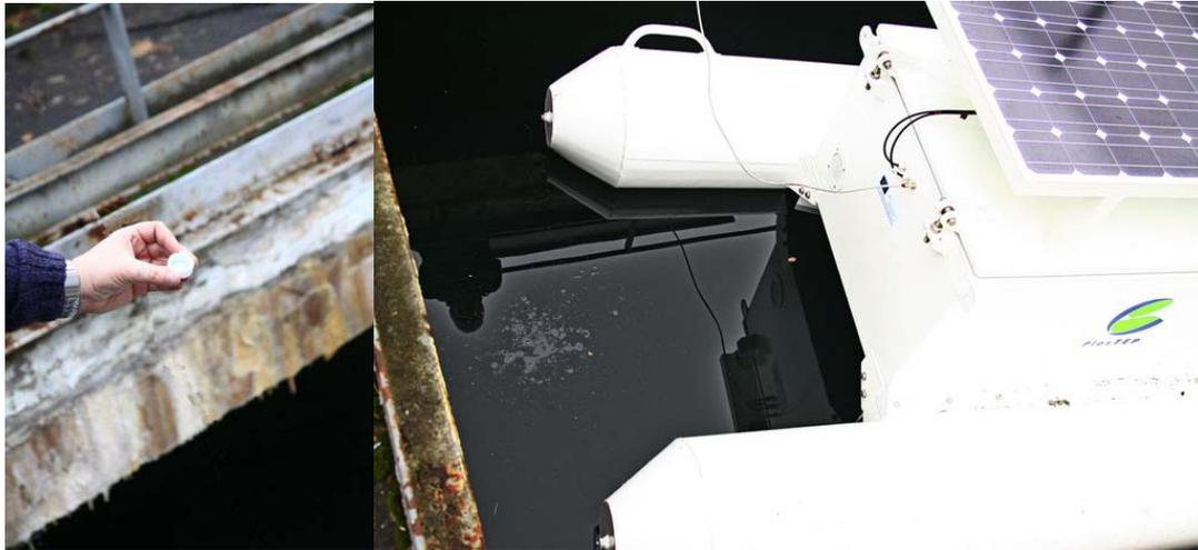
Fig. 6. Sloping 15 ml of kerosene onto the water surface in front of the plasma device.
