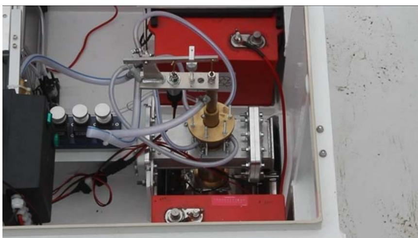
Fig. 3. Igniter on the microwave plasma module.
