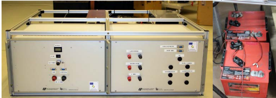
Fig. 2. Optimised power supply module with batteries ready for the final device.
