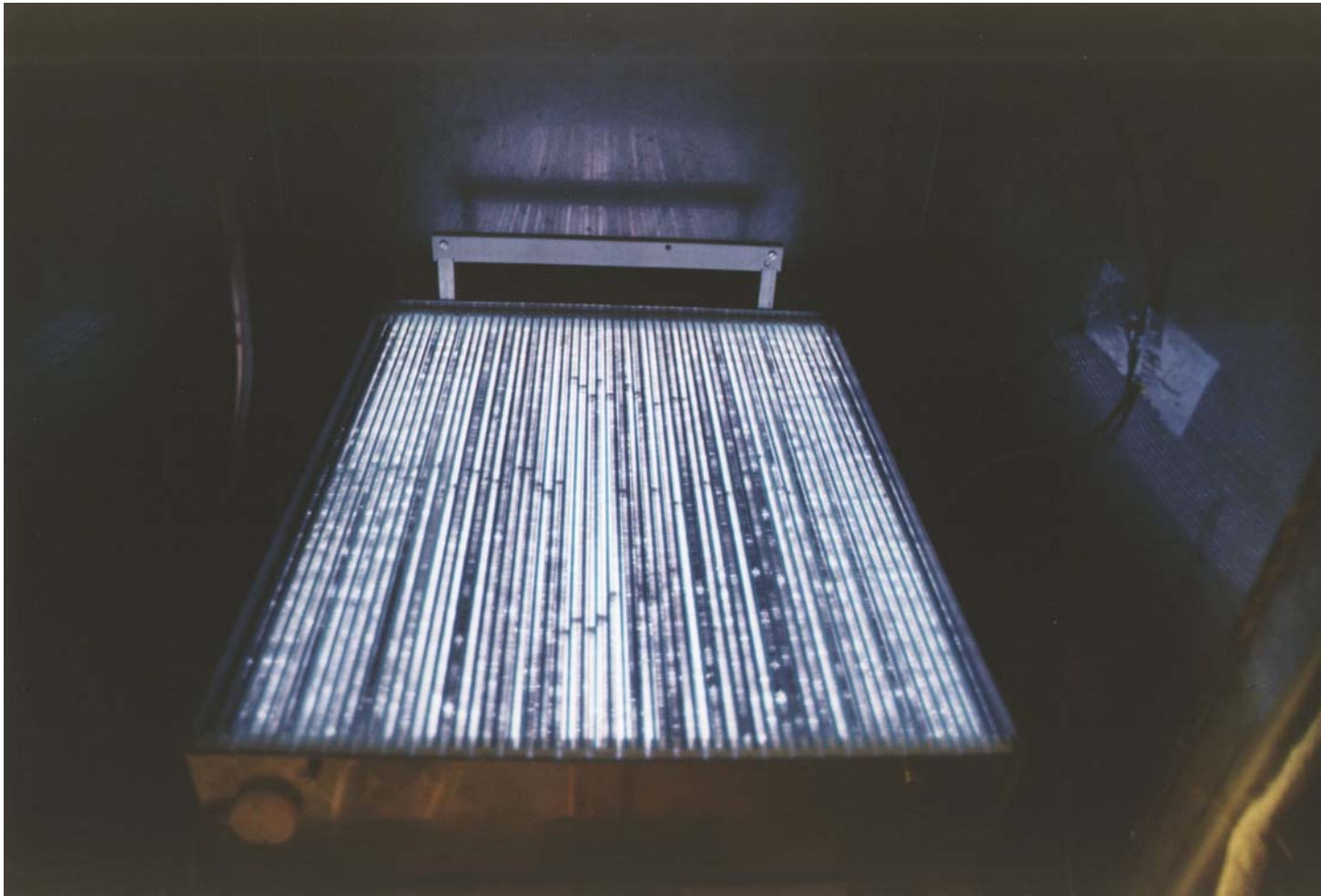
Figure 3: NTP module with glass barriers in operation
